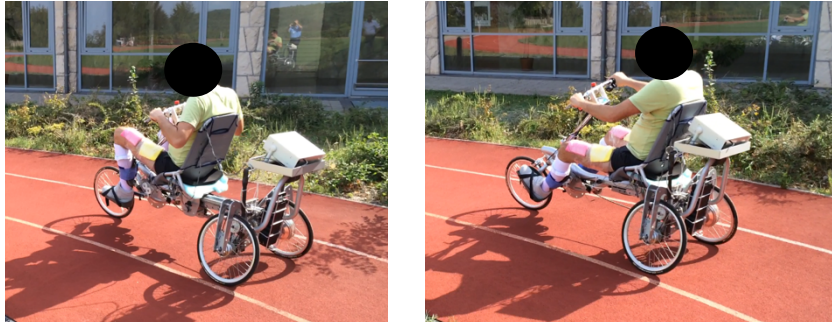
Fig 2: Left: Bilateral knee extension starts and actively drives the tricycle as the quadriceps muscles are stimulated; Right: The end of quadriceps stimulation (start of "rowing mode").
